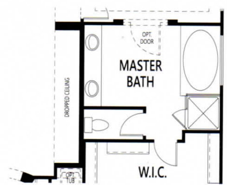
9 DROP-IN TUB AT MASTER BATH
