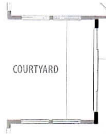
12ft Sliding Glass Doors at Courtyard
