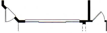
12ft. Multi-Sliding Glass Doors at Great Room
